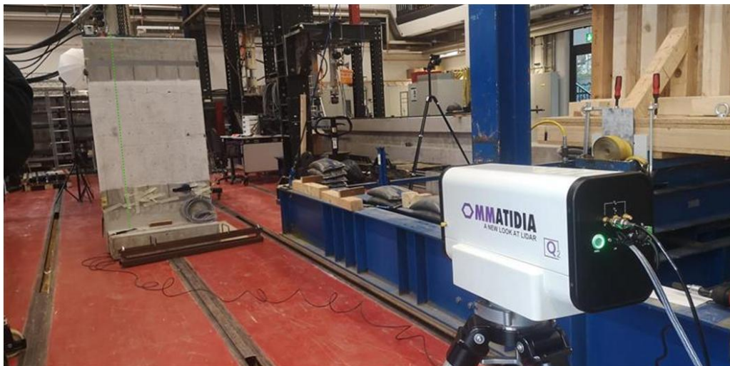
Figure 3: Experimental setup for the concrete slab at the Institute of Structural Mechanics at the Bauhaus-Universität Weimar ( https://www.uni-weimar.de/en/civil-and-environmental-engineering/institute/ism/ ). The green dashed line is a superimposed guide to the eye to show how the frames are measured.
