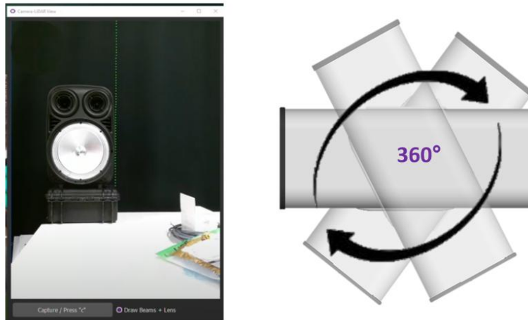
Figure 2: left: field view from Q2. The green dotted line represents the 65 measuring points. Right: by scanning the azimuthal angle, the full-field view measurement is obtained
